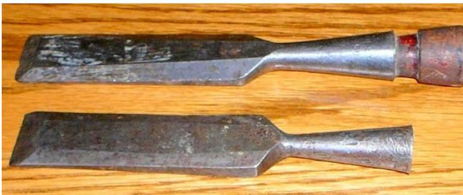
Socketed chisels are usually larger, very stout chisels, meant to be struck with a mallet. The socket prevents the end of the handle from splitting apart, and only gets tighter as it is struck with the mallet.
